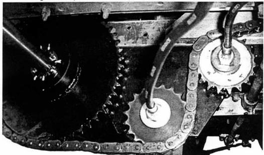
sprocket so that it is exactly aligned with the forward sprocket on the transmission. The eight Allen headed screws were gradually tightened in a crisscross pattern and then torqued them to 12.3 foot pounds. A paint stripe applied to the "PowerLock" and axle can be used to detect any slippage.
